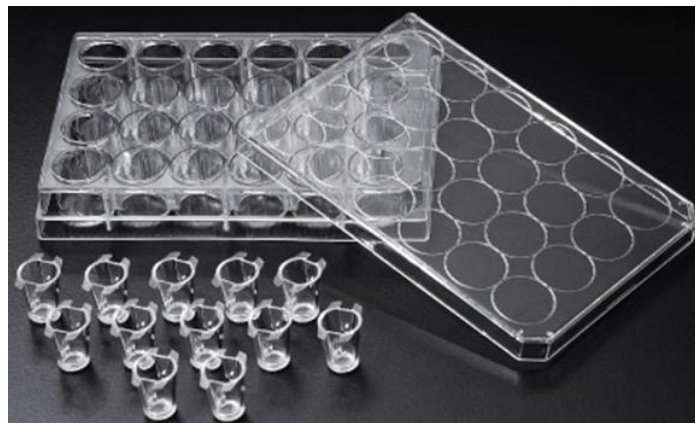
Figure 9. Cell culture inserts with a corresponding 24 well plate. Pores at the bottom membrane of cell inserts allow medium flow while flanges on the insert rim facilitate handling (downloaded from www.biolab.com ).
