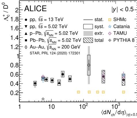
**Fig. 4.** The  $p_T$ -integrated and to  $p_T > 0$  extrapolated  $\Lambda_c^+ / D^0$  ratios in central and mid-central Pb–Pb collisions at  $\sqrt{s_{NN}} = 5.02$  TeV compared to the same ratio at pp and p–Pb [11,32] and Au–Au [34] multiplicities. Predictions from theoretical calculations are shown as well [7,8,10,23,30,31].
