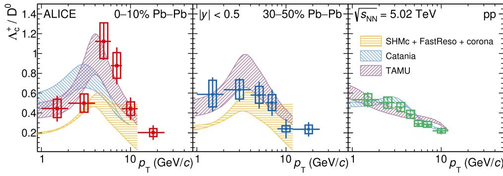
**Fig. 3.** The  $\Lambda_c^+/D^0$  yield ratio as a function of  $p_T$  in 0–10% (left) and 30–50% (middle) Pb–Pb and pp (right) collisions at  $\sqrt{s_{NN}} = 5.02$  TeV compared with predictions of different theoretical calculations [7,8,10,30,31,64].
