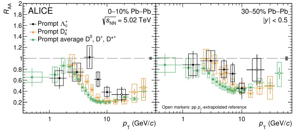
**Fig. 2.** Nuclear modification factor  $R_{AA}$  of prompt  $\Lambda_c^+$  baryons in central (0–10%; left) and mid-central (30–50%; right) Pb–Pb collisions at  $\sqrt{s_{NN}} = 5.02$  TeV, compared with the  $R_{AA}$  of prompt  $D_s^+$  [60] and the average of prompt non-strange D mesons [56]. The normalization uncertainties are shown as boxes around unity.
