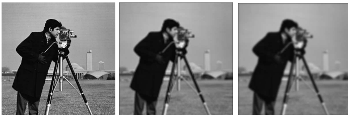
(a) Slika kamermana. (b) 'average'; r = c = 10 (c) 'gaussian'; r, c = 25; \sigma = 4
