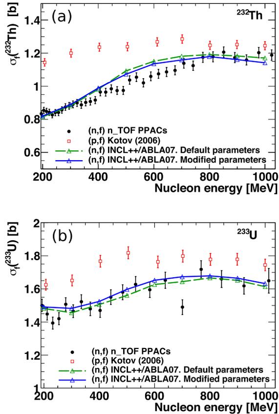
FIG. 15. Our results on neutron-induced fission cross sections for  $^{232}\text{Th}$  (a) and  $^{233}\text{U}$  (b) are shown together with the calculated values from the combination of reaction codes INCL++ and ABLA07. Proton-induced data from Ref. [72] are also shown for comparison.
