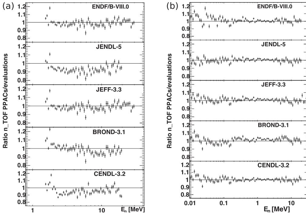
FIG. 13. Ratios between our data and evaluations from the major libraries [1–3,68,69] for the fission cross section ratios  $\sigma_f(^{232}\text{Th})/\sigma_f(^{235}\text{U})$  (a) and  $\sigma_f(^{233}\text{U})/\sigma_f(^{235}\text{U})$  (b).
