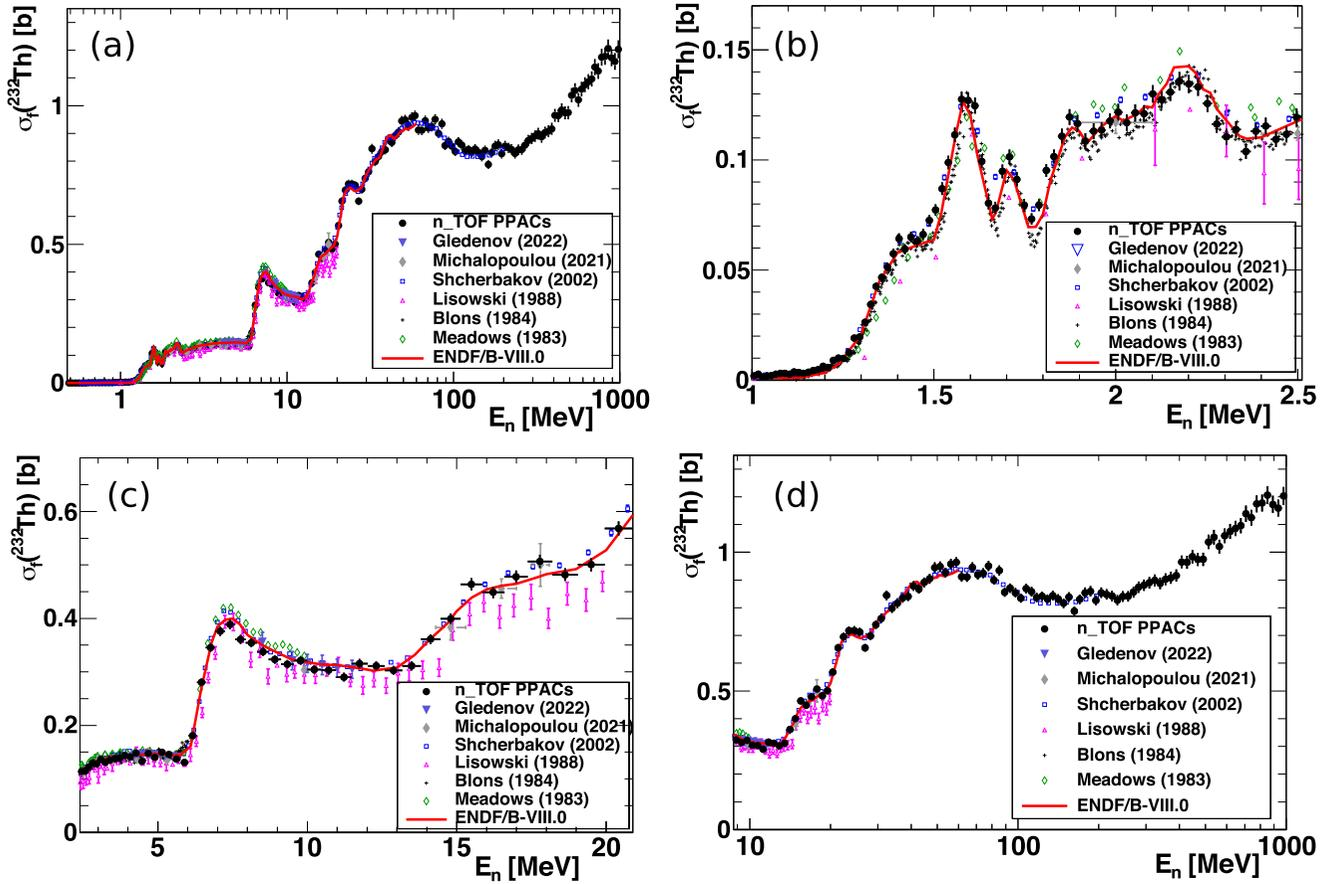
FIG. 10. The final cross section of  $^{232}\text{Th}(n, f)$  obtained in the present work is compared with previous results available in the EXFOR database [54,56–60] and with the ENDF/B-VIII.0 evaluation [1]. The full energy range is shown in (a). For clarity, detailed views covering different energy ranges are shown in separate panels: (b) shows the threshold for first-chance fission, while the second-chance fission threshold is displayed in (c); the high energy range can be seen in (d).
