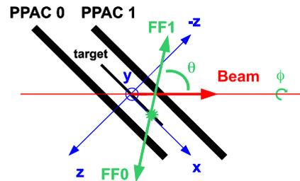
FIG. 2. Reference system used to calculate the emission angle  $\theta$  of the fission fragments (FFs) in Phase 2, where PPACs and targets are tilted  $45^\circ$  with respect to the neutron beam direction. Fission fragments emitted at every possible value of  $\theta$  between  $0^\circ$  and  $90^\circ$  can be detected. See Ref. [20] for a more detailed description.
