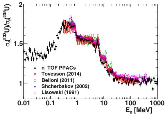
FIG. 11. Fission cross section ratio of  $^{233}\text{U}$  relative to  $^{235}\text{U}$  from 10 keV up to 1 GeV, compared with previous results [54,56,63,64]. The error bars in our data represent statistical uncertainties.
