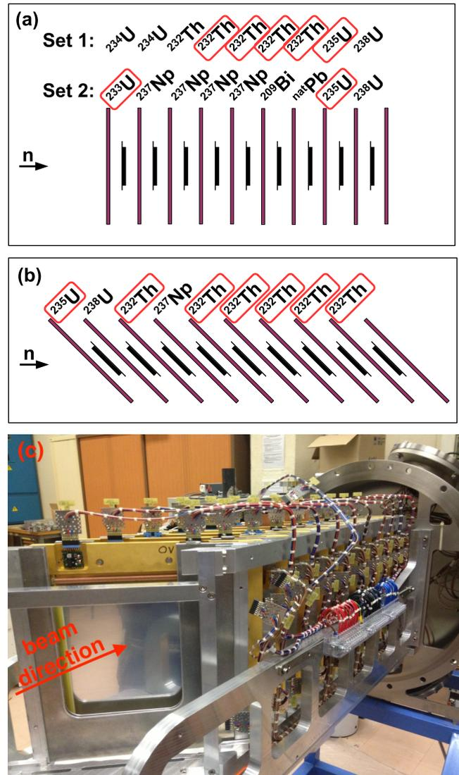
FIG. 1. Schematic views (not to scale) of the PPAC detectors and the targets used during Phase 1 (a) and Phase 2 (b). The targets studied in this work are indicated by the red rectangles. A photo of the stack of PPACs and targets used in Phase 2 can be seen in (c), where the arrow follows the neutron beam direction, and points to the aluminized electrode of the first PPAC. The active area of each PPAC is  $20 \times 20 \text{ cm}^2$ .
