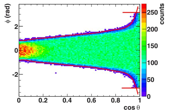
FIG. 6. Detection efficiency of the tilted setup (Phase 2) as a function of the emission angles  $\theta$  and  $\phi$ , according to GEANT4 simulations. The red lines represent the contour used to calculate the total efficiency. More details about the detection efficiency on this setup can be found in Ref. [20].
