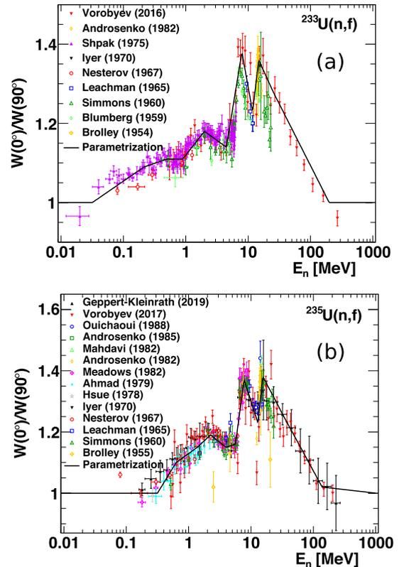
FIG. 4. Experimental values of the anisotropy parameter  $A = W(0^\circ)/W(90^\circ)$  for the neutron-induced fission of  $^{233}\text{U}$  (a) [23–31] and  $^{235}\text{U}$  (b) [24,26–29,32–40] retrieved from EXFOR, as a function of the neutron energy. The solid lines represent the parametrizations of the anisotropy used in this work.
