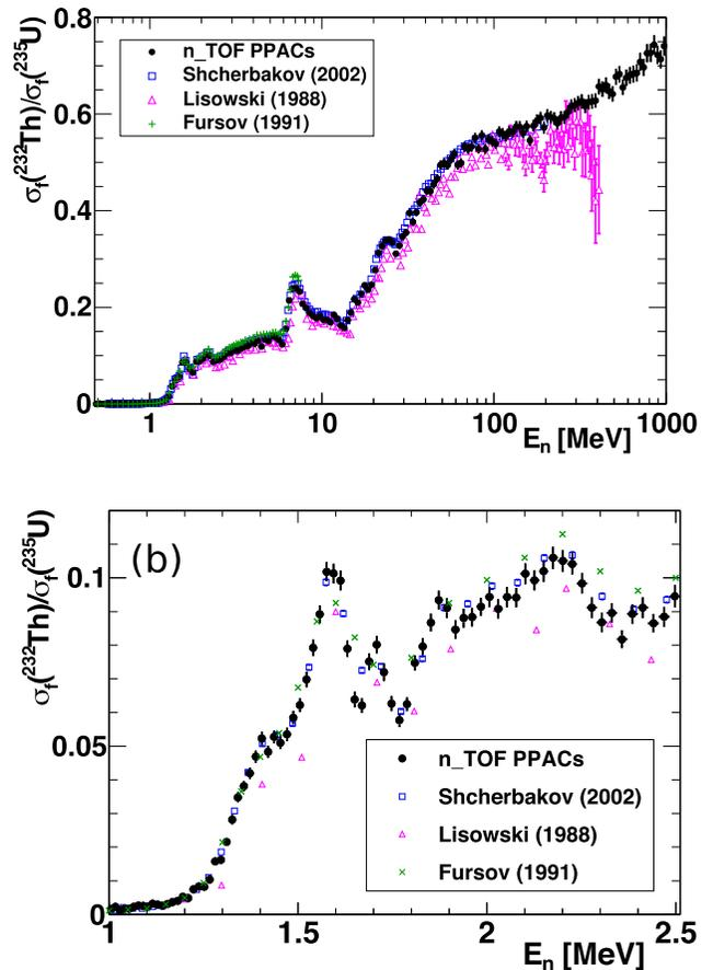
FIG. 9. Fission cross section ratio of  $^{232}\text{Th}$  relative to  $^{235}\text{U}$ , compared with previous results [54–56]. Panel (b) shows a detailed view around fission threshold of the full range in (a). The error bars in our data represent statistical uncertainties.
