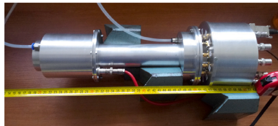
Fig. 3. Picture of the multi-section ionization chamber with connectors, two gas pipes and HV cable. The design of set-up ensures gas flow between the detector housing with electrodes and the part located in the immediate vicinity of the box with preamplifiers.
