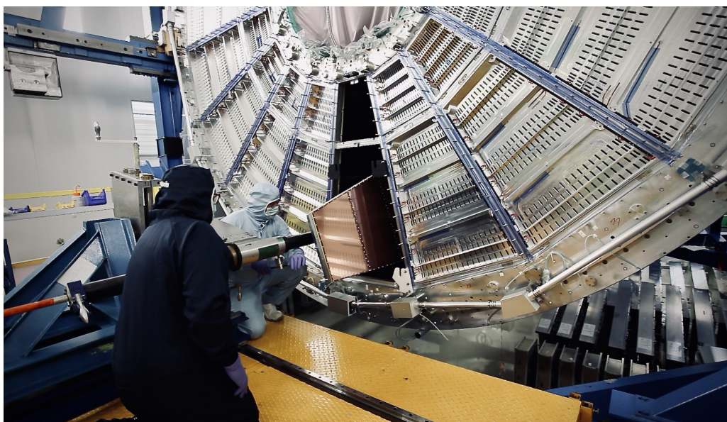
Figure 46. Installation of an OROC mounted on the mounting tool, which in turn stands on the elevating platform. The uninstalled MWPCs are stored underneath the TPC in TT-boxes, visible in the lower right corner.
