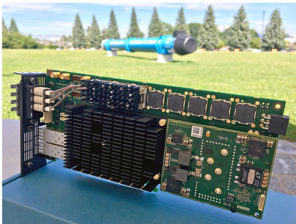
Figure 6. Picture of a CRU; bottom left, FPGA cooling radiator, bottom right, power mezzanine; top row; 3 out of 8 Minipods installed; top left, fiber optics cable to MPO connector on front panel; bottom left, SFP transceivers.
