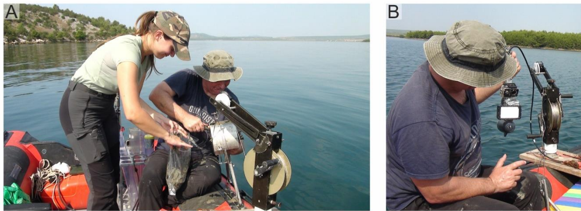
Figure 4.4 A. Grab sediment collection with Van Veen grab. B. Seafloor observations with SeaViewer underwater drop camera.
