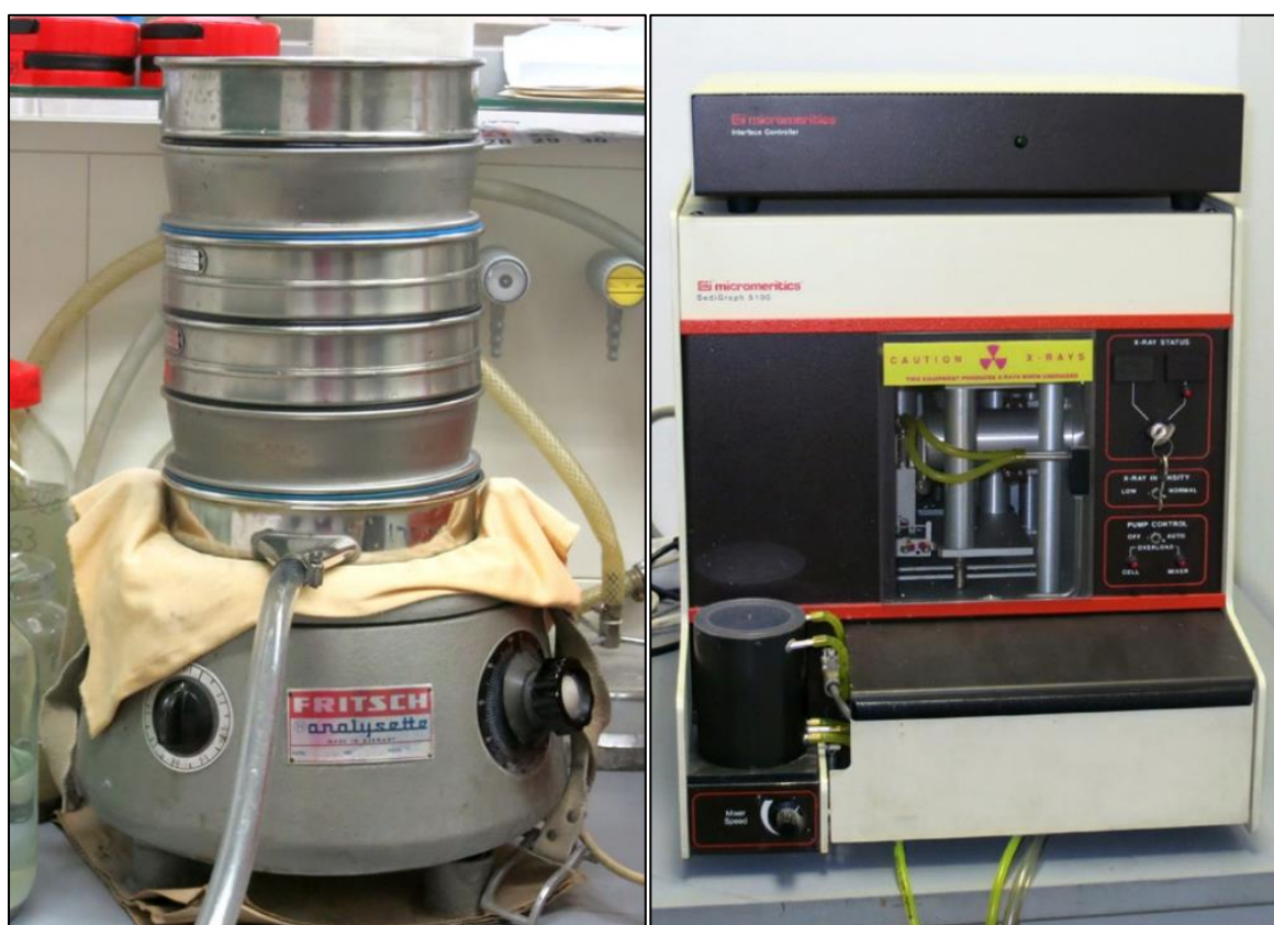
Figure 4.6. Wet sieving and sedigraph method for determining grain size in sediment (Division for Geology and Paleontology, Department of Geology, Faculty of Science, Zagreb).
