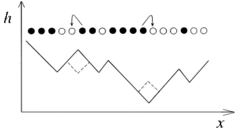
Figure 2.3: Mapping of ASEP to the model of surface growth by ballistic deposition. In ASEP, particle movements to the right or left correspond to increase or decrease in surface height,  $h_i \rightarrow h_i + 2$  or  $h_i \rightarrow h_i - 2$ , respectively.
