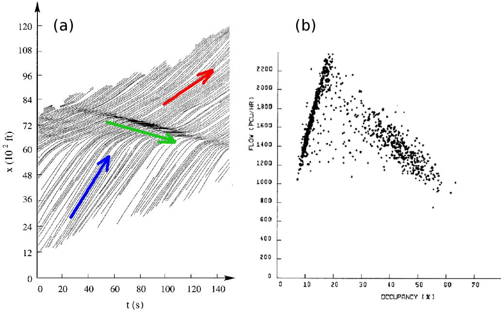
Figure 2.6: (a) Trajectories of cars photographed from air and their corresponding velocity vectors (denoted by red and blue arrows); notice a “phantom” traffic jam travelling backwards, its velocity vector being denoted by green arrow. (b) Fundamental diagram of real traffic, taken from [55].
