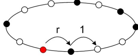
Figure 4.1: Schematic picture of TASEP with a static defect from which the particles move with reduced probability  $0 < r < 1$ . The probability of hopping from other sites is 1.
