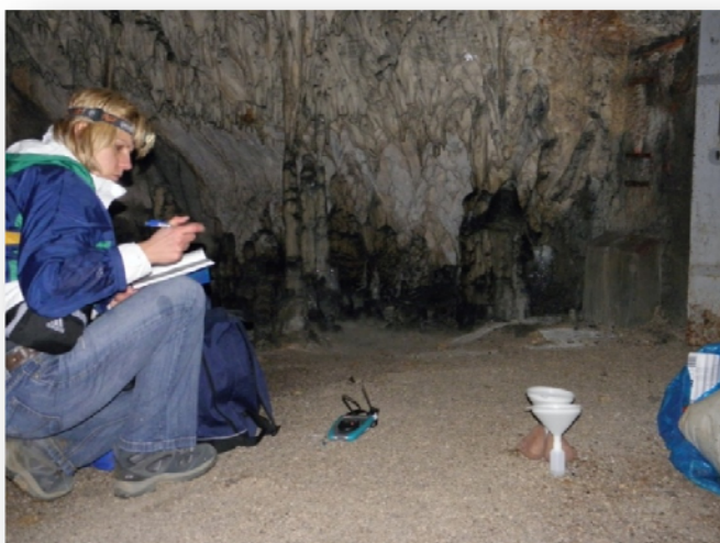
Figure B.5 Sampling of drip water and measurement of field parameters. Logging of field data into sampling diary
