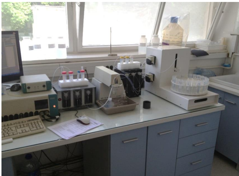
Figure 3.14. Automated voltammetric system for trace metals analysis
