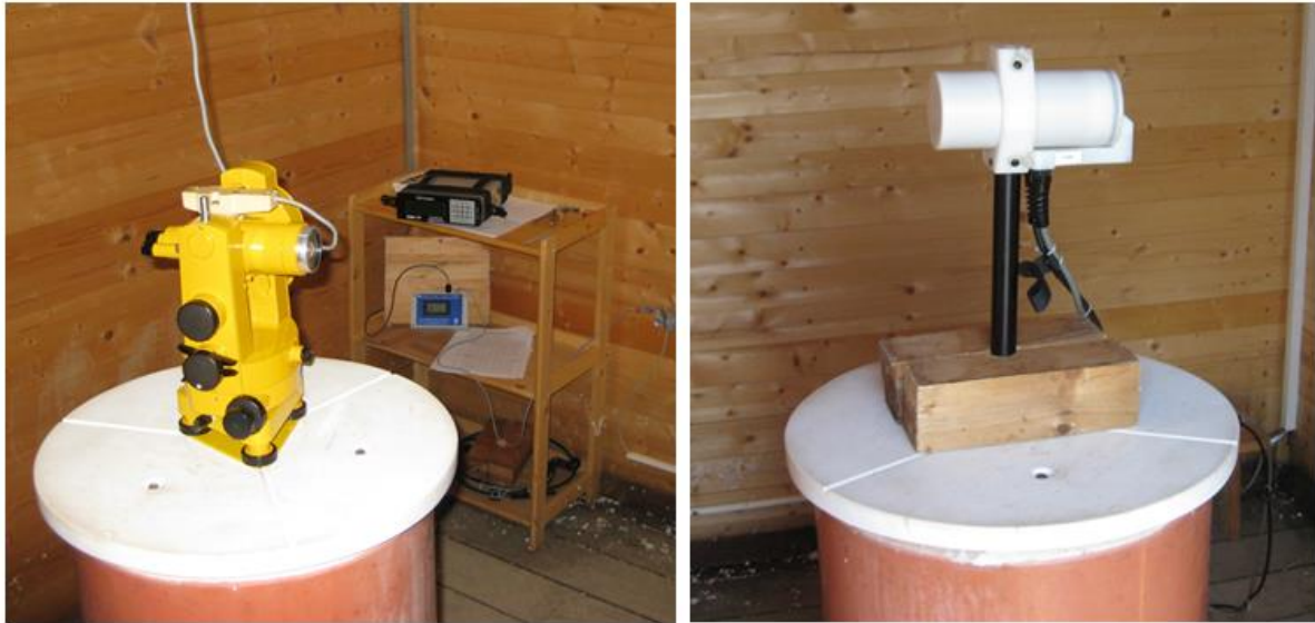
Figure 2.2 Absolute instruments operating at LON. Left: DI-flux magnetometer (manufacturer: MinGeo, Hungary). It is based on a Zeiss 010A nonmagnetic theodolite and equipped with a DI fluxgate magnetometer (Model G, manufacturer: DMI). Right: Overhauser proton precession GSM-19F magnetometer (manufacturer: GEM Systems, Canada).
