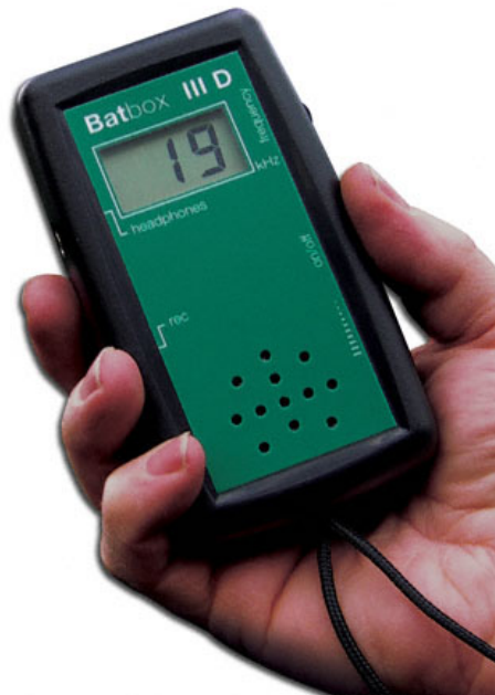
Batbox heterodyne bat detektor
