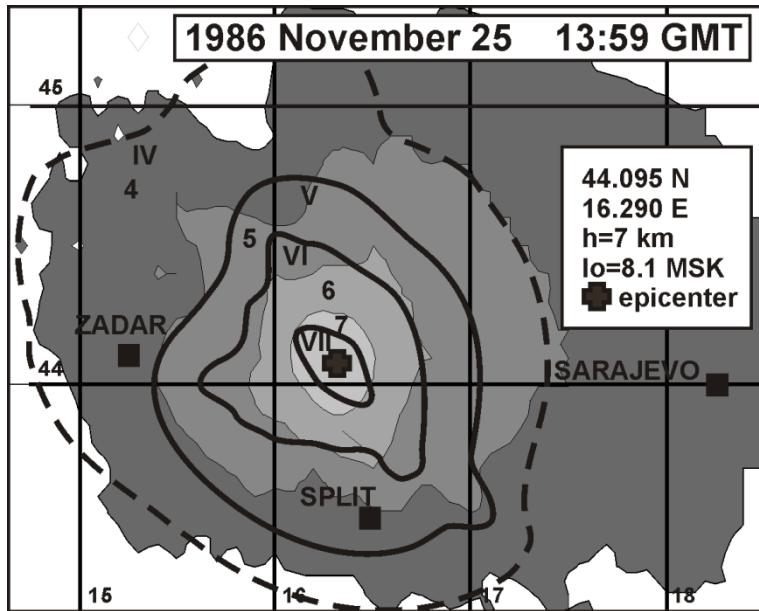
**Figure II.** Model (shaded areas and Arabic numerals) and empirical (dashed lines and Roman numerals) isoseismals 25th of November 1986 M=5.5 earthquake with epicenter near Knin. The results for all grid points are shown, although the macroseismic field for the sea area does not exist. Coast line and islands are not displayed.
