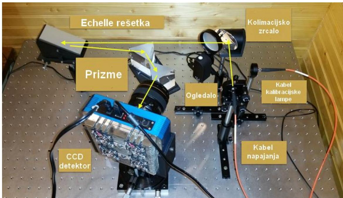
Slika 30: IRES Echelle rešetke. (Intermediate Resolution Echelle Spectrometer) [17]
