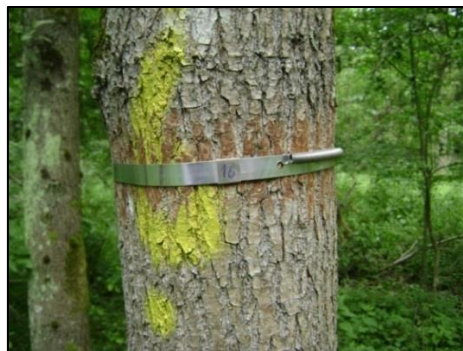
Figure 2.6: Tree with installed dendrometer band
