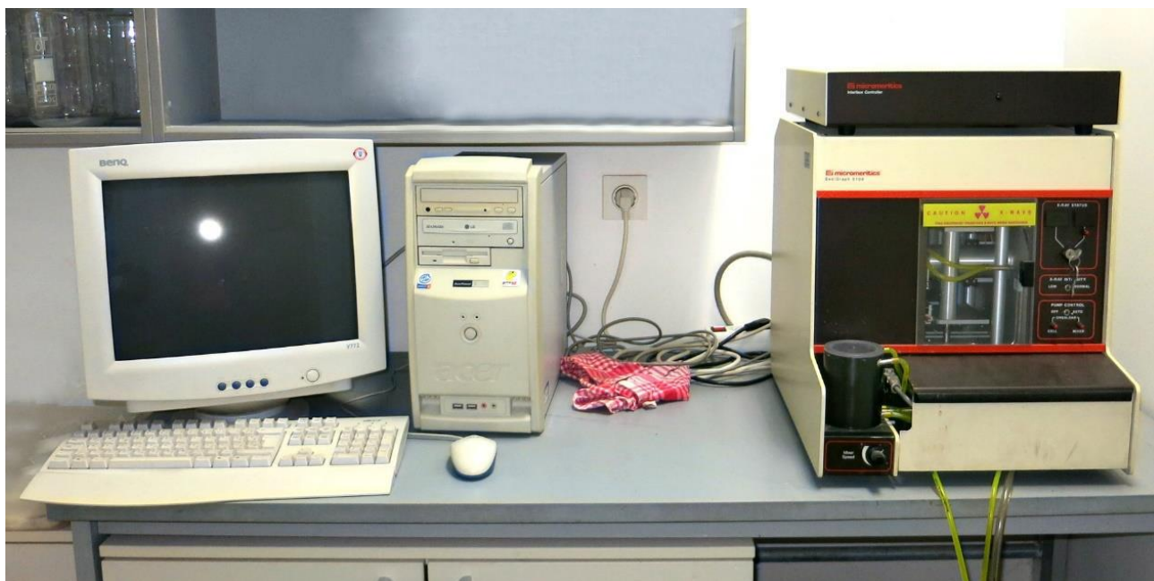
Slika 9. SediGraph 5100 (Micromeritics Instrument Corporation), Geološko-paleontološki zavod PMF-a. Pikelj (2018)
