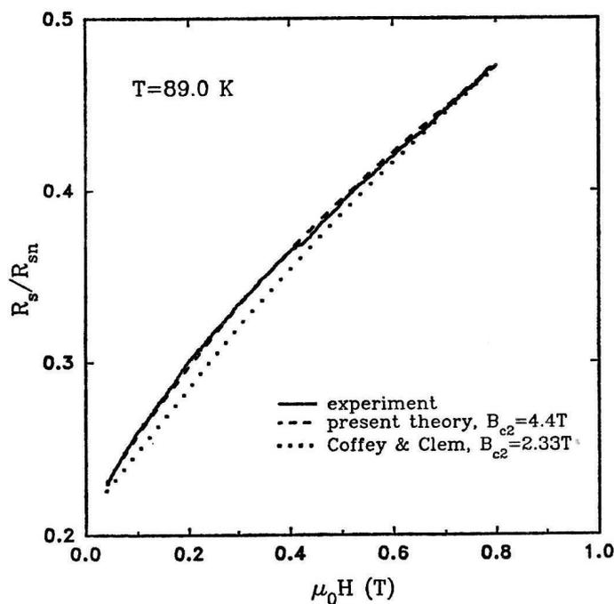
Fig. 3. Comparison of the experimental curve of  $R_s/R_{sn}$  at  $T = 89.0$  K with the theoretical forms of  $R_s/R_{sn}$  using effective conductivities: a)  $1/\sigma_{\text{eff}}$  of Eq. (5) with  $\omega \gg \omega_0$  (dashed line,  $B_{c2} = 4.4$  T), b)  $(1/\sigma_{\text{eff}})_{CC}$  as explained in text (dotted line,  $B_{c2} = 2.33$  T).
