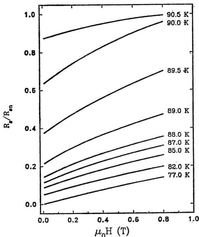
Fig. 2. Theoretical curves for the normalized surface resistance calculated using the effective conductivity of Eq. (5) with variable  $B_{c2}$  in order to find the best fit to the corresponding experimental curves in Fig. 1. The fitting parameters  $B_{c2}$  for the curves from top to bottom are (in Tesla): 1.0, 1.1, 2.2, 4.4, 7.2, 8.9, 11.4, 14.9 and 18.5.
