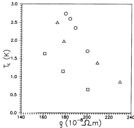
Fig. 4. Plot of the superconducting transition temperature  $T_c$  vs. resistivity for ○—  $(\text{Zr}_{0.67}\text{Co}_{0.33})_{1-x}\text{H}_x$ , △—  $(\text{Zr}_{0.67}\text{Ni}_{0.33})_{1-x}\text{H}_x$  and □—  $(\text{Zr}_{0.7}\text{Cu}_{0.3})_{1-x}\text{H}_x$  metallic glasses.
