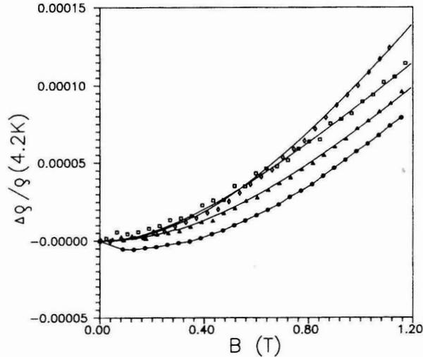
Fig. 3. Magnetoresistivity of  $(\text{Zr}_{0.68}\text{Fe}_{0.32})_{1-x}\text{H}_x$  at  $T = 4.2$  K:  $\circ$  -  $x = 0$ ;  $\triangle$  -  $x = 0.017$ ;  $\square$  -  $x = 0.066$ ;  $\diamond$  -  $x = 0.077$ . Solid lines are the best fits of the WL and EI expressions (Ref. 4).
