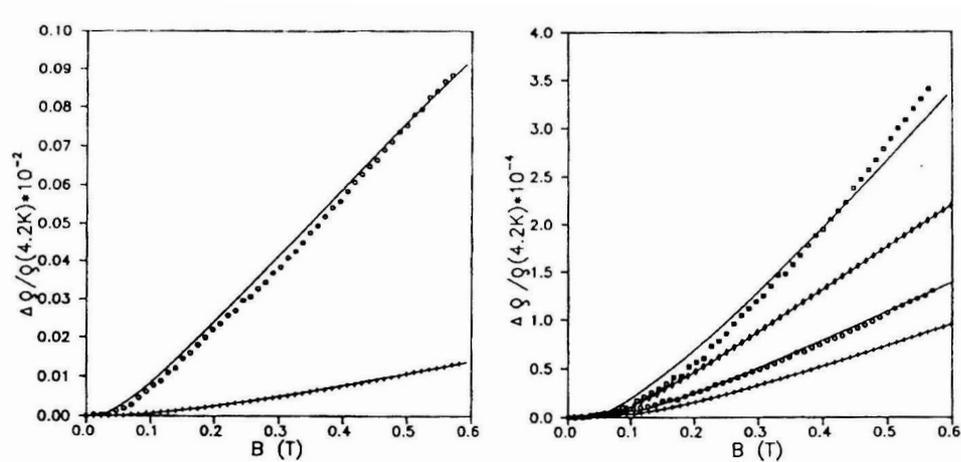
Fig. 1. Magnetoresistivity of  $(\text{Zr}_{0.67}\text{Co}_{0.33})_{0.952}\text{H}_{0.048}$  at  $T = 2.7$  K ( $\circ$ ), and  $T = 4.2$  K ( $+$ ). Solid lines are the best fits of the WL and EI expressions (Ref. 4).
