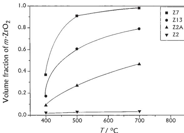
Figure 5. The  $m$ -ZrO<sub>2</sub> volume fraction of starting samples Z13, Z7, Z2 and Z2A as a function of temperature.
