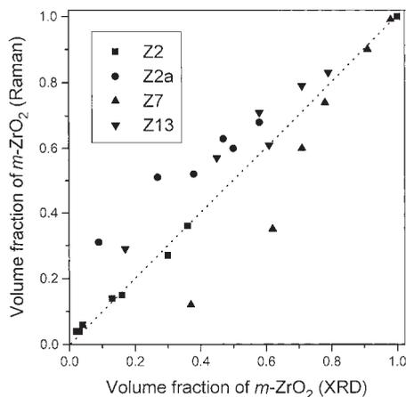
Figure 11. The relation between the  $m$ -ZrO<sub>2</sub> volume fraction determined by laser Raman spectroscopy using the method proposed by Clarke and Adar<sup>18</sup> and the  $m$ -ZrO<sub>2</sub> volume fraction determined by XRD using the method proposed by Toraya.<sup>17</sup>
