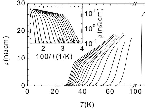
Fig. 1. Resistive transitions in  $B = 0, 1, 1.5, 2, 3, 4, 5, 6, 7, 8, 9, 10, 11, 12, 13, 14$  and  $15 \text{ T}$  (right to left) for the Bi2223/Ag tape. The inset: Arrhenius plot of the  $\rho(T, B)$  dependence for the same fields without  $B = 0$  (left to right).
