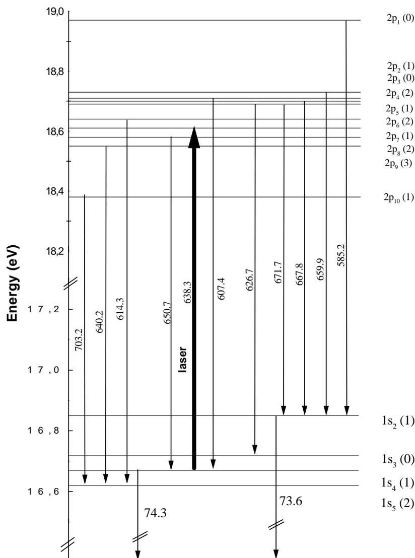
Fig. 3. Partial term diagram of Ne I.
