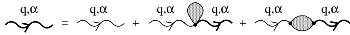
Fig. 1. The Dyson equation for the photon Green function. The bare second-order (first-order) electron-photon coupling leads to the second (third) term on the right-hand side, giving rise to the diamagnetic (current-current) contribution to the photon self-energy.
