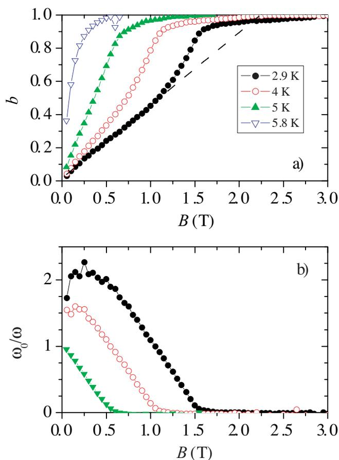
FIG. 4. (Color online) Parameters  $b$  and  $\omega_0/\omega$  of the effective conductivity model extracted from the data of Fig. 3. The dashed line shows the extrapolation of the linear section at  $T=2.9\text{ K}$ .
