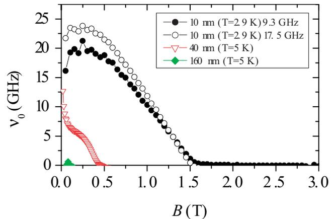
FIG. 6. (Color online) Field dependence of the depinning frequency  $\nu_0 = \omega_0/2\pi$  obtained by driving frequency 9.3 GHz for three niobium films at  $T/T_c \approx 0.5$ : 10 nm film at 2.9 K (black full circles); 40 nm film at 5 K (red opened triangles) and 160 nm film at 5 K (green full diamonds). The depinning frequency obtained by driving frequency 17.5 GHz for the 10 nm film at 2.9 K is shown by open black circles.
