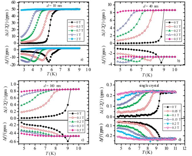
FIG. 2. (Color online) Measured temperature dependence of complex frequency shift of four niobium samples: (a) thin film  $d = 10$  nm; (b) thin film  $d = 40$  nm; (c) thin film  $d = 160$  nm; (d) single crystal. The driving frequency was 9.3 GHz. Applied perpendicular static magnetic fields are indicated in the legends.
