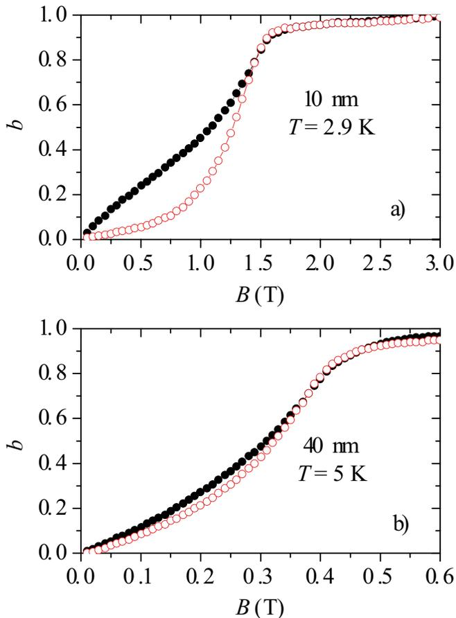
FIG. 5. (Color online) Comparison of  $b$  obtained by full inversion of complex frequency shift (full black circles) and  $b$  obtained from absorption measurement alone under the assumption that depinning frequency is much lower than driving frequency (red open circles): (a) 10-nm film at 2.9 K; (b) 40-nm film at 5 K.
