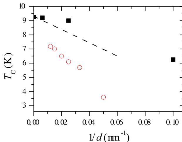
FIG. 1. (Color online) Thickness dependence of the transition temperature of the measured niobium films (full squares). The data are compared with clean samples of Wolf *et al.* (Ref. 24) and Kodama *et al.* (Ref. 25) (dashed line), and with dirty samples of Minhaj *et al.* (Ref. 26) (circles).
