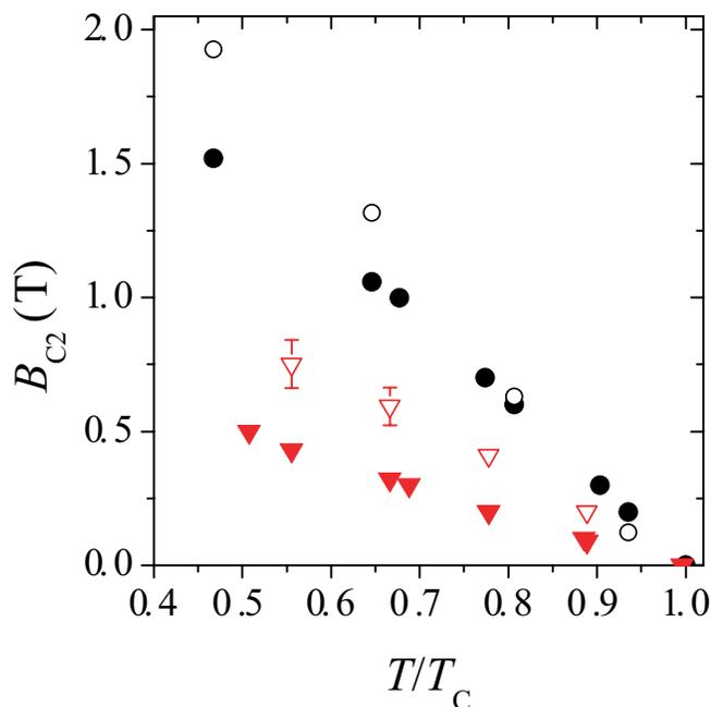
FIG. 7. (Color online) Upper critical field  $B_{c2}$  of the 10-nm film obtained by the 90% criterion from the microwave absorption measurements (black full circles). Upper critical field  $B_{c2}^*$  of the same sample obtained from the linear section of  $b$  (black opened circles). The same is shown for the 40-nm film by red triangles.
