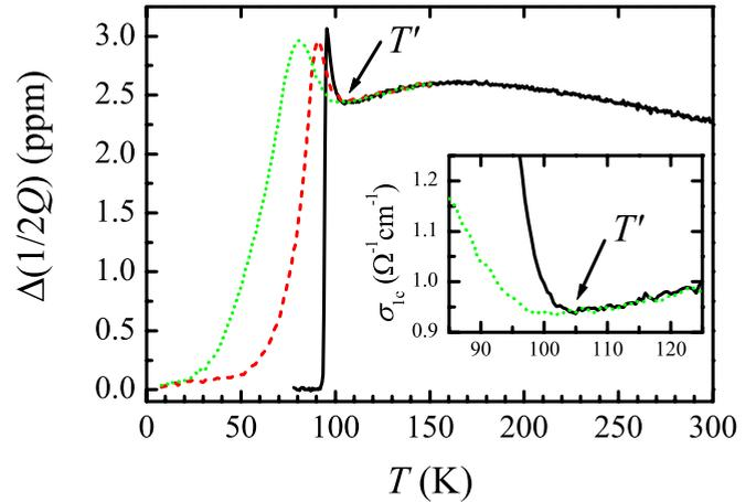
FIG. 3. (Color online) Microwave absorption measured with the external dc magnetic field applied in the  $c$  direction, in the same geometry as in the case of Fig. 2(b). The applied fields were 0, 3, and 8 T, plotted in full (black), dashed (red) and dotted (green) lines, respectively. Inset: temperature dependence of  $c$ -axis conductivity calculated from the microwave absorption data for zero field (full black line) and for 8 T (dotted green line).
