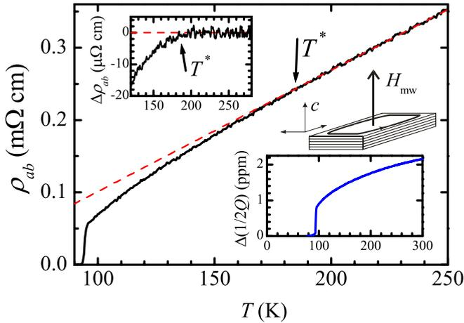
FIG. 1. (Color online) Temperature dependence of  $\rho_{ab}$  in the single crystal of nearly optimally doped  $\text{HgBa}_2\text{CuO}_{4+\delta}$  (full line) calculated from the measured microwave absorption (lower inset, with  $H_{\text{mw}} \parallel c$ ). The dashed line represents extrapolated linear behavior above 200 K. Upper inset: difference between  $\rho_{ab}$  and the linear behavior extrapolated to low  $T$  clearly reveals  $T^*$ .
