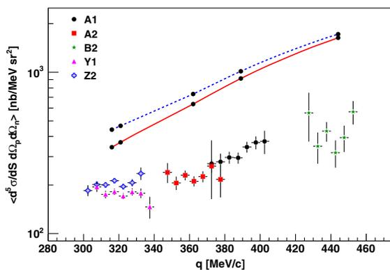
FIG. 3 (color online). The  ${}^3\text{He}(e, e'pn)$  reaction cross section shown as a function of  $q$  for  $50 \leq p_m \leq 100$  MeV/c and  $235 \leq \omega \leq 265$  MeV. Results from different kinematic settings are shown by the different types of markers for the data points. The line convention is the same as in Fig. 2. The theoretical cross section was calculated at the points indicated by the black circles.
