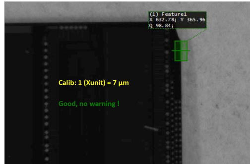
Figure 3.6: Image of the visual inspection of a chip corner. The camera scans the edge of the chip. The position of the camera is indicated by the square with the target cross visible on the top right. The image has been taken just before the machine reaches the broken corner, thus no error is yet indicated.
