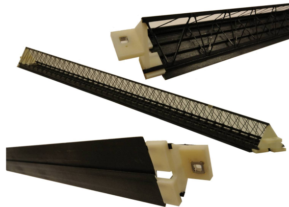
(b) ITS outer Stave prototype.
