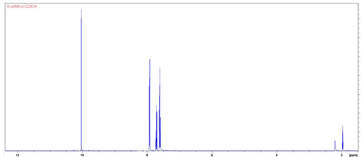
Slika D31. Spektar  $^1\text{H}$  NMR standarda benzaldehida ( $\gamma = 5,0 \text{ mg mL}^{-1}$ ) snimljen u acetonitrilu-*d*3 pri 25 °C.
