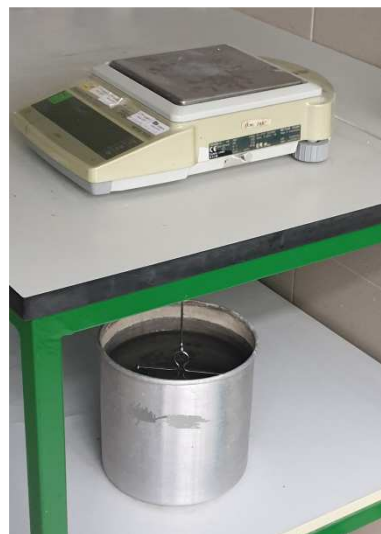
Figure 3.14. The balance for the weighing under the water
