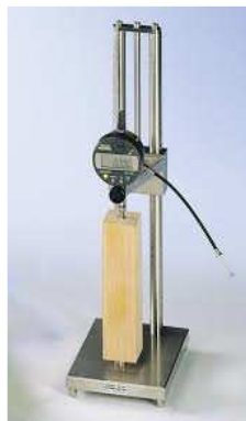
Figure 3.13. Instrument for dimensional stability determination
