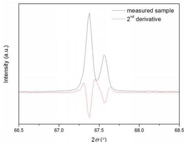
Figure 9. The original LaB<sub>6</sub> profile and its 2<sup>nd</sup> derivative.
