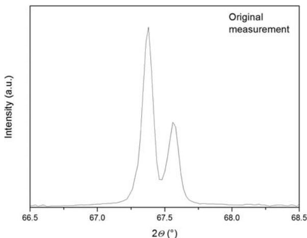
Figure 8. X-ray diffraction of the LaB<sub>6</sub> sample (around 67.5°).
