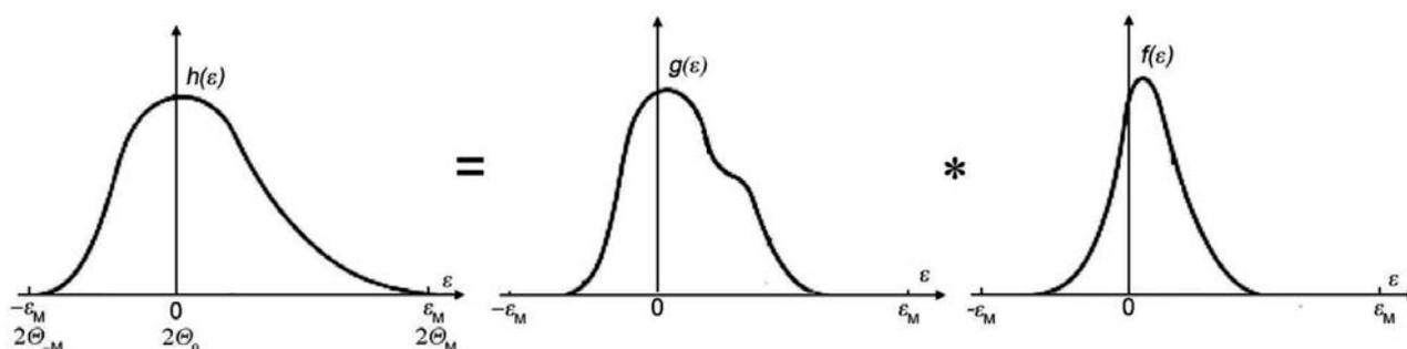
Figure 1. Observed, pure diffraction and instrumental profile.
