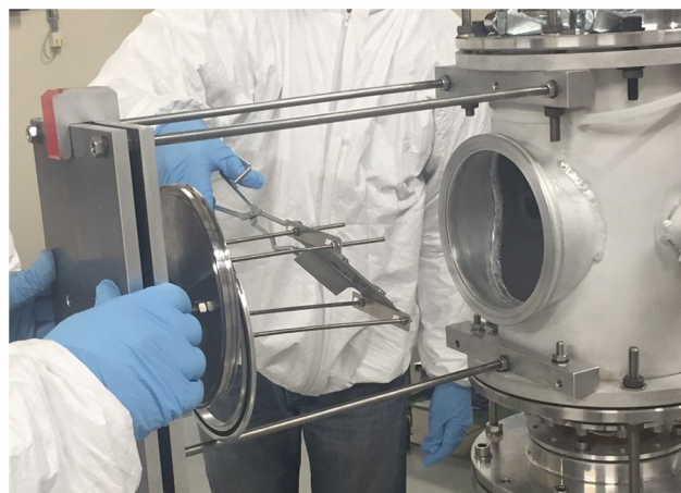
Fig. 5. Insertion of the ^7\text{Be} radioactive target in the setup, with a support independent of the telescope detector installed from the opposite side of the chamber.
