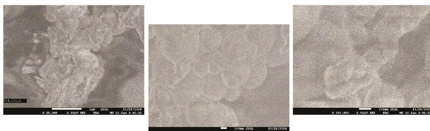
**Figure 3.** SEM images of Fe<sub>2</sub>B/SiO<sub>2</sub> particles.
