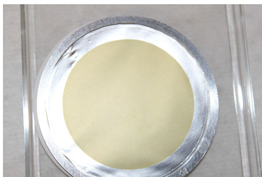
Fig. 34 A ^{233}\text{U} deposit with an areal density of 220\ \mu\text{g}/\text{cm}^2 and a diameter of 40 mm prepared by molecular plating on a 0.01 mm thick aluminium foil glued onto an aluminium ring
