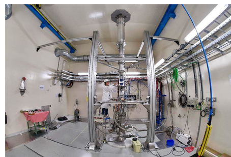
Fig. 9 A photo of the second experimental area (EAR-2), with detectors mounted along the vertical beam-line
