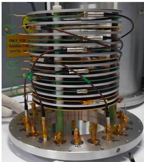
**Fig. 23** A setup consisting of ten Micromegas detectors, coupled with six  $^{241}\text{Am}$  samples and two  $^{235}\text{U}$  and  $^{238}\text{U}$  reference samples, before insertion into the chamber
