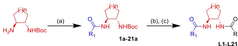
**Slika 42.** (a) TBTU, HOBr, DIPEA, R<sub>1</sub>-COOH, CH<sub>2</sub>Cl<sub>2</sub>, 2 dana, s.t.; (b) TFA/CH<sub>2</sub>Cl<sub>2</sub>, 1 h, s.t.; (c) TBTU, HOBr, DIPEA, R-COOH, CH<sub>2</sub>Cl<sub>2</sub>, 2 dana, s.t.; n = 1 ili 2.
