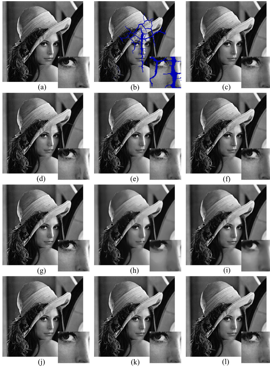
Fig. 5. Inpainted gray scale Lena using different PDE based inpainting methods with 2.5\times zoom over the nose and right eye region. (a) Original image, (b) Image with the inpainting domain in blue, (c) Matlab inpaintn function, (d) Transport equation of Bertalmio, (e) Local Laplace inpainting, (f) Local biharmonic inpainting, (g) Integer order CHTE, (h) TV inpainting, (i) TV4 inpainting, and fractional order CHTE with (j) \mu = 0.7 , (k) \mu = 0.8 , (l) \mu = 0.9 .
