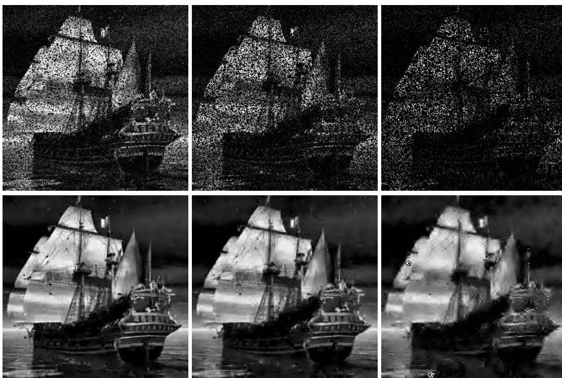
Figure A.4: Inpainting results of the image Ship . The figure shows the given images (top) and their inpainting results (bottom), for 25% missing pixels (left), 50% missing pixels (center) and 75% missing pixels (right).
