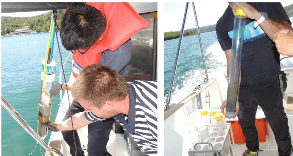
**Figure 4.2.** Sediment sampling using Uwitec gravity corer
