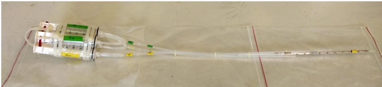
**Figure 4.9.** The homemade device for recovering supernatant water at three depths from the SWI (2 cm, 5 cm and 15 cm)
