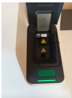
Slika 2.27: Utor za kivete instrumenta Zetasizer Ultra (Malvern Panalytical)
