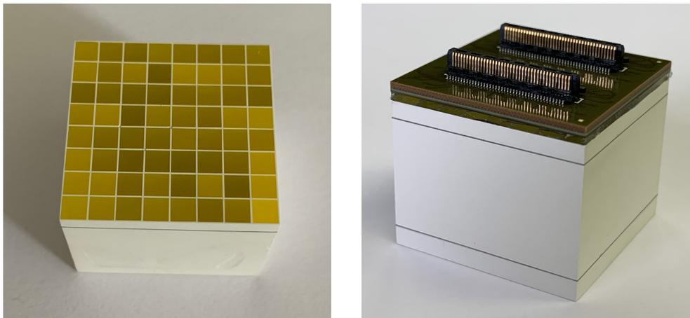
**Figure 1.** GaGG:Ce matrix containing 64 crystals with a size of  $3 \text{ mm} \times 3 \text{ mm} \times 20 \text{ mm}$  in  $8 \times 8$  configuration. All crystal sides were polished and casted in 0.2 mm of white epoxy (**left**). GaGG:Ce matrix along with the SiPM array optically coupled with a silicon optical interface (**right**).
