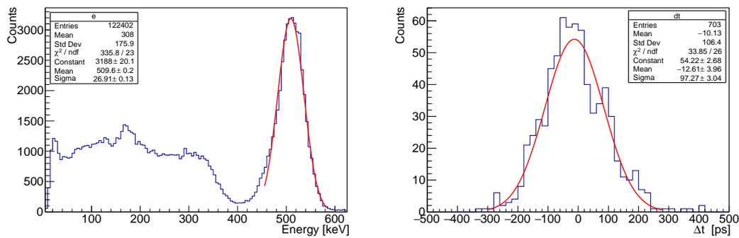
**Figure 3.** The 511 keV gamma spectrum obtained by  $3 \times 3 \times 3$  mm<sup>3</sup> LYSO crystal with KETEK SiPM at 4 V overvoltage (left). Coincidence time spectrum of annihilation gammas from <sup>22</sup>Na, detected by two  $3 \times 3 \times 3$  mm<sup>3</sup> LYSO crystals with KETEK SiPM at 4V overvoltage (right). Events with energy within 511 keV  $\pm 1 \sigma$  were selected.
