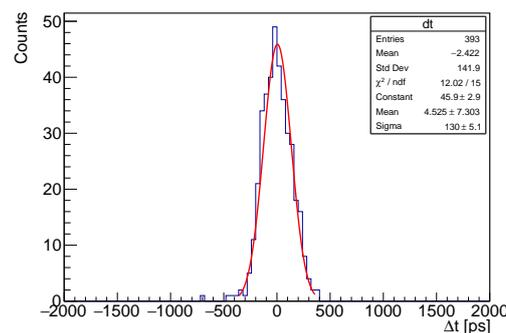
**Figure 6.** Coincidence time spectrum of annihilation gammas from  $^{22}\text{Na}$ , detected by a  $3 \times 3 \times 3$  mm<sup>3</sup> LYSO crystal and a crystal from GaGG Module II operating at  $V_{OV} = 4$  V.
