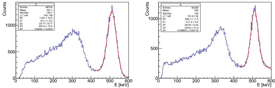
**Figure 4.** The spectra of 511 keV gammas from  $^{22}\text{Na}$  measured by a crystal from Module I at  $V_{OV} = 4$  V (left) and from Module II at  $V_{OV} = 3$  V (right). The fit function is the one given in Equation (3). The spectra with the best obtained energy resolutions are shown:  $\Delta E/E = 10.9\%$  for the Module I and  $\Delta E/E = 9.2\%$  for the Module II.
