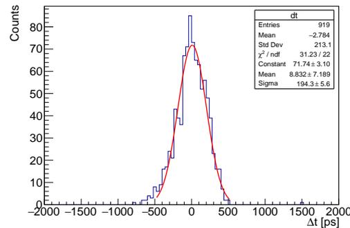
**Figure 5.** Coincidence time spectrum of annihilation gammas from  $^{22}\text{Na}$ , detected by a  $3 \times 3 \times 3$  mm<sup>3</sup> LYSO crystal and a crystal from GaGG Module I operating at  $V_{OV} = 4$  V.
