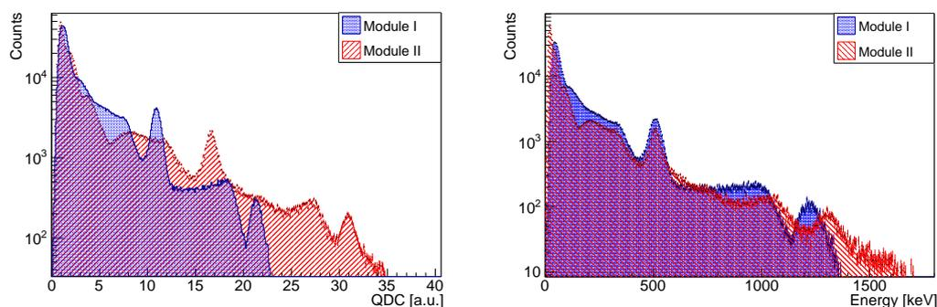
**Figure 2.** The  $^{22}\text{Na}$  spectra before non-linearity correction and calibration measured by a crystal from Module I and Module II at  $V_{OV} = 3$  V, respectively (**left**). The energy spectra of  $^{22}\text{Na}$  after applying the non-linearity correction and calibration of the 511 keV peak (**right**).
