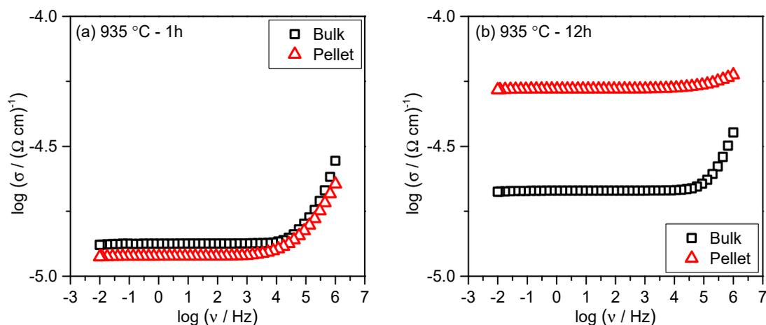
**Figure 6.** Comparison of the conductivity spectra measured at 30 °C for glass-ceramics prepared from the bulk glass (black squares) and pelleted glass powder (red triangles) at 935 °C for (a) 1 h and (b) 12 h.
