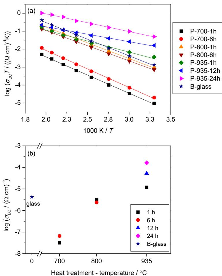
**Figure 5.** (a) Arrhenius plot of the parent 60WO<sub>3</sub>-40P<sub>2</sub>O<sub>5</sub> glass and glass-ceramics prepared from pellets and (b) their DC conductivity,  $\sigma_{DC}$ , at 30 °C as a function of crystallization temperature and time. The error bars are at most of the order of the symbol size.
