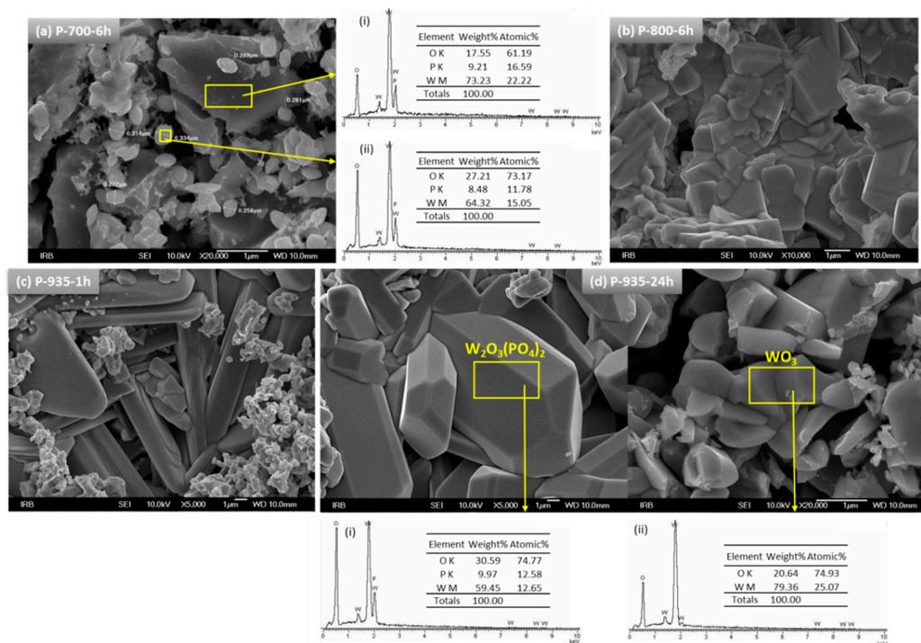
**Figure 3.** SEM micrographs of glass-ceramics prepared at (a) 700 °C for 6 h, (b) 800 °C for 6 h, (c) 935 °C for 1 h, and (d) 935 °C for 24 h. EDS spectra and tables with chemical composition from selected areas of the samples are shown in the insets (i) and (ii).
