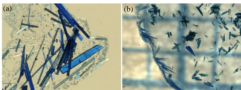
Slika 19. Prikaz kristala: a) spoja  $[\text{Cu}(\text{Gly})(\text{H}_2\text{O})(\text{phen})]_2\text{SO}_4 \cdot 6\text{H}_2\text{O}$  različite morfologije (iglice i pločice) i b) spoja  $[\text{Cu}(\text{Gly})(\text{H}_2\text{O})(\text{phen})]_2\text{SO}_4 \cdot 8\text{H}_2\text{O}$  različite morfologije (plave iglice i pločice) i  $[\text{Cu}(\text{ox})(\text{H}_2\text{O})(\text{phen})] \cdot \text{H}_2\text{O}$  (zeleno-plavi kristali)
