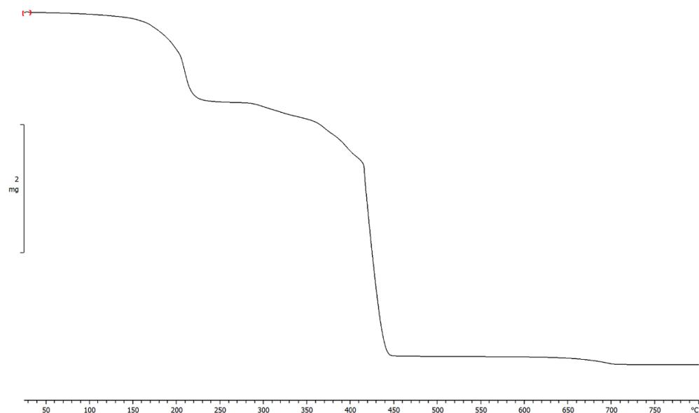
Slika D21. TG krivulja spoja  $\{[\text{Cu}(\text{Gly})(\text{H}_2\text{O})(\text{phen})][\text{Cu}(\mu\text{-Gly})(\text{phen})]\text{SO}_4 \cdot 2\text{H}_2\text{O}\}_n$
