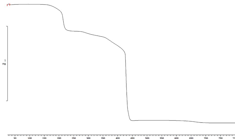
Slika D22. TG krivulja produkta raspada spoja  $[\text{Cu}(\text{Gly})(\text{H}_2\text{O})(\text{phen})]_2\text{SO}_4 \cdot 6\text{H}_2\text{O}$
