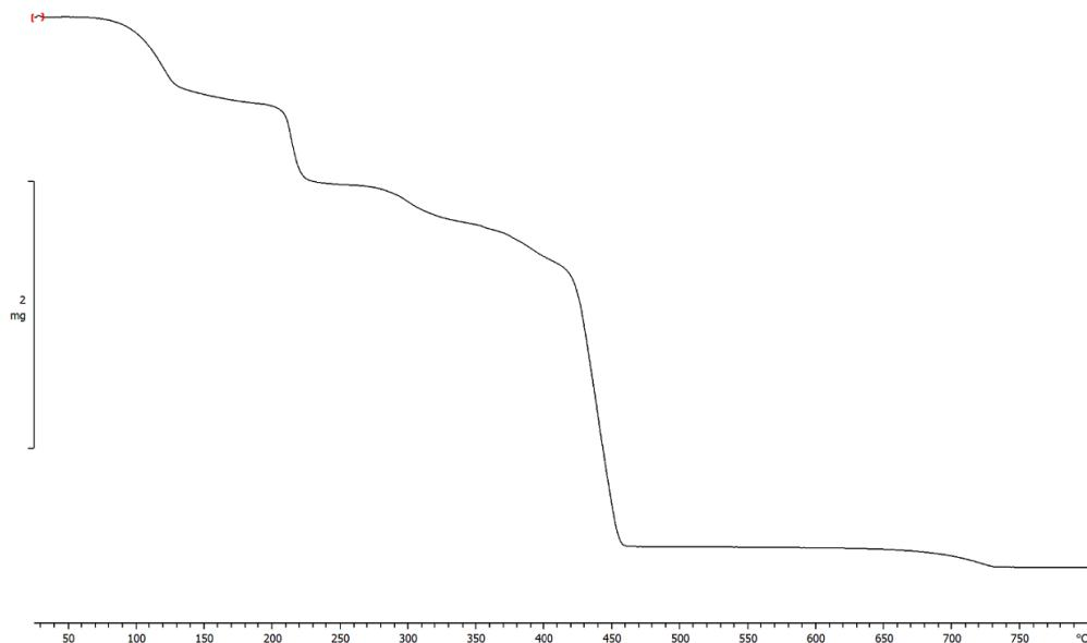
Slika D20. TG krivulja spoja  $[\text{Cu}(\text{Gly})(\text{H}_2\text{O})(\text{phen})][\text{Cu}(\text{Gly})\text{SO}_4(\text{phen})] \cdot 5\text{H}_2\text{O}$
