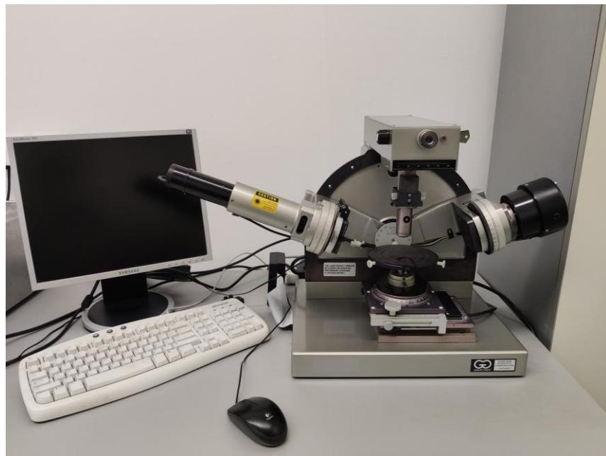
Slika 15. Elipsometar *Gaertner Scientific Ellipsometer L116B-USB*
