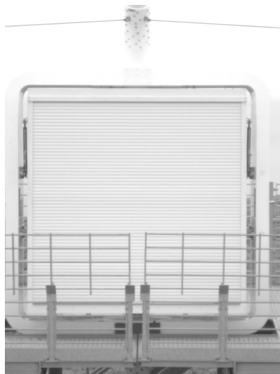
(a) Image of the PMT camera taken by CDM during the day. The shutter is closed to protect the PMTs.
