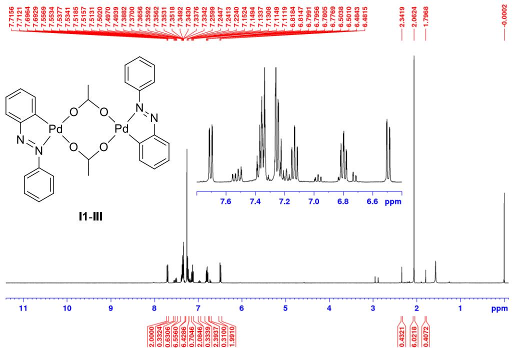
**Slika D169.**  $^1\text{H}$  NMR spektar I1-III u  $\text{CDCl}_3$  (400 MHz).
