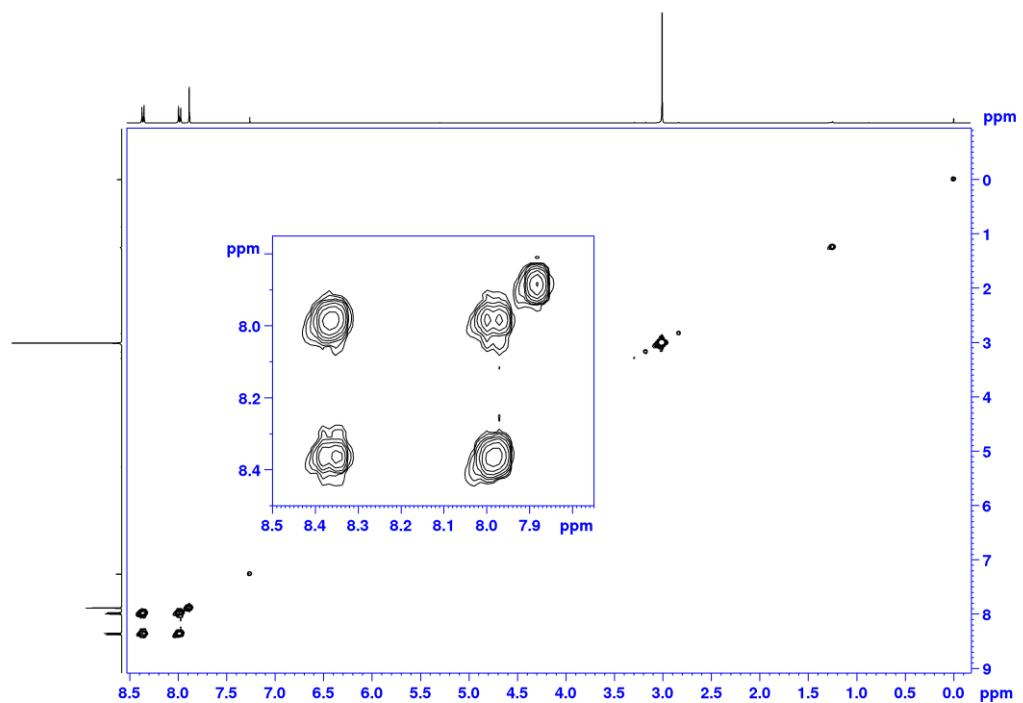
Slika D149. COSY spektar L8Cl-IV u  $\text{CDCl}_3$  (400 MHz).
