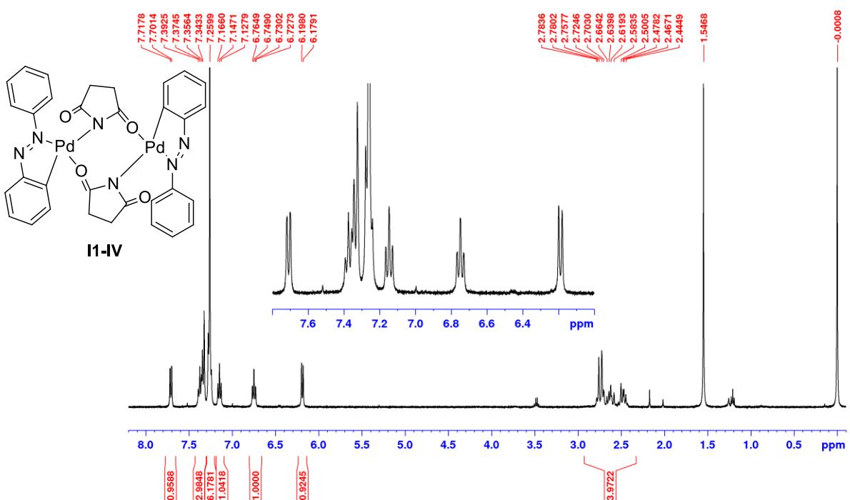
**Slika D170.**  $^1\text{H}$  NMR spektar I1-IV u  $\text{CDCl}_3$  (400 MHz).
