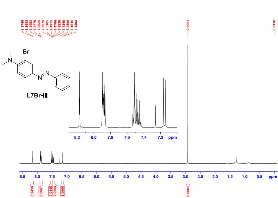
**Slika D132.**  $^1\text{H}$  NMR spektar L7Br-III u  $\text{CDCl}_3$  (400 MHz).
