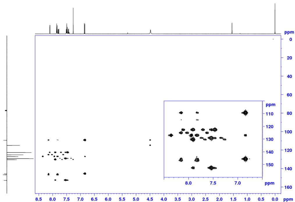
**Slika D121.** HMBC spektar L6Br-III u  $\text{CDCl}_3$  (400 MHz).
