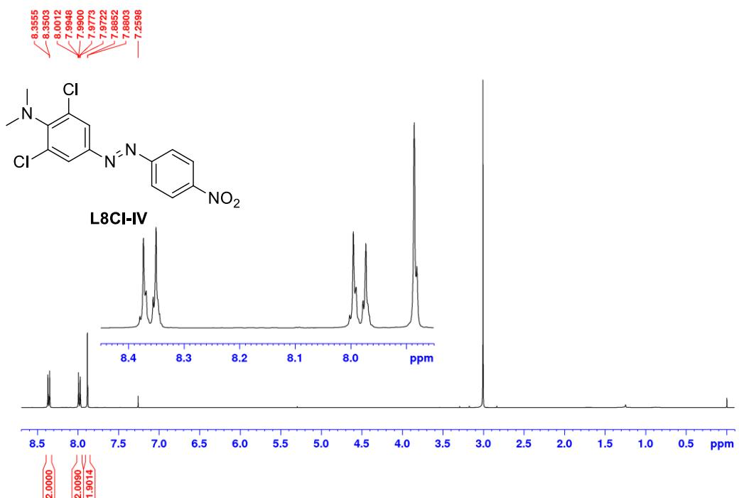
**Slika D147.**  $^1\text{H}$  NMR spektar L8Cl-IV u  $\text{CDCl}_3$  (400 MHz).
