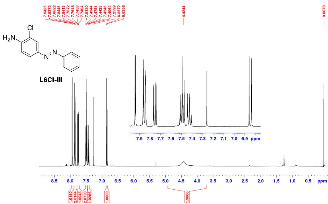
**Slika D112.**  $^1\text{H}$  NMR spektar **L6Cl-III** u  $\text{CDCl}_3$  (400 MHz).
