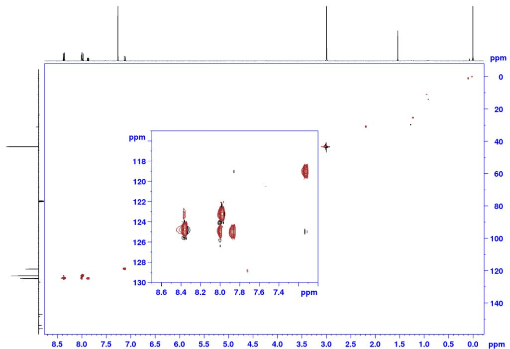
Slika D145. HSQC spektar L8Cl-III u  $\text{CDCl}_3$  (400 MHz).
