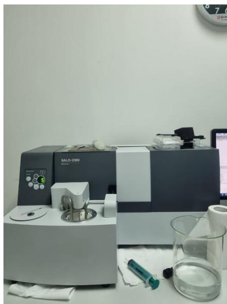
Slika 9. Laserski difraktometar Shimadzu Laser Diffraction Particle Size Analyzer
