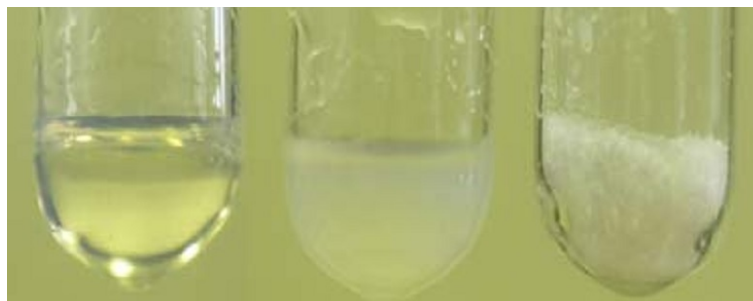
Figure 2.1: Phases of cholesteryl benzoate. Liquid (left), liquid crystalline (middle) and solid (right) phase of cholesteryl benzoate [30].
