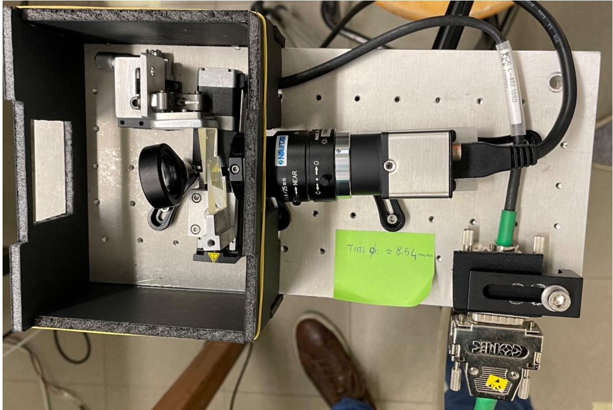
Figure 4.10 Image of the TWINS interferometer with wedges, translator stages and CCD camera for use in macroscopic objects such as art paintings.
