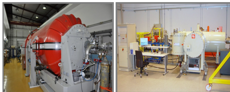
Figure 4.6: 6.0 MV EN Tandem Van de Graaf accelerator on the left and 1.0 MV Tandetron accelerator on the right.[5]
