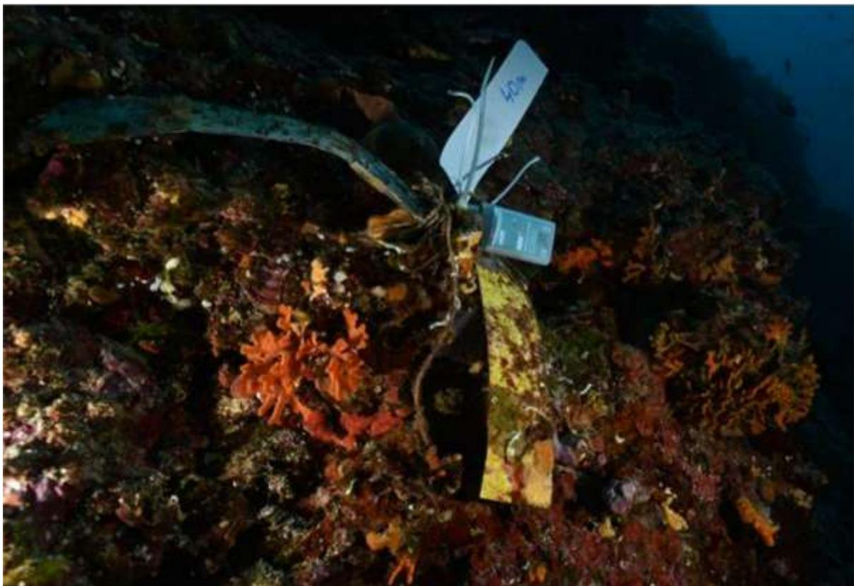
**Slika P1.** Mjerač temperature mora (Onset Computers data logger).
